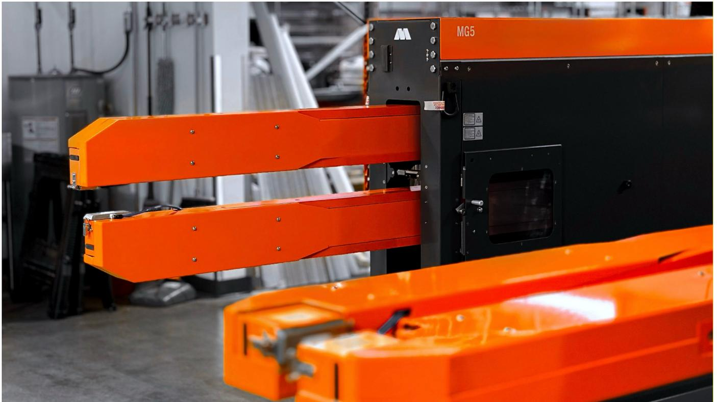
Sensors scan across the material at a sampling rate of 1-5 kHz. The thickness is determined from the distance of both measuring heads to each other and the difference of the measured individual distances to the material to be measured.
