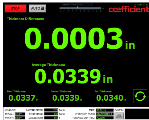
Large Numerical Display, Including Thickness Difference
