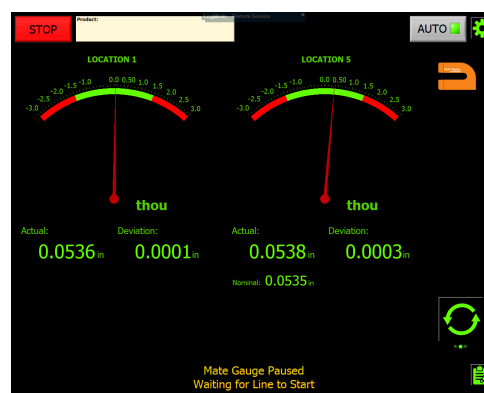
Needle Gauge Location Showing Left-Right thickness.
