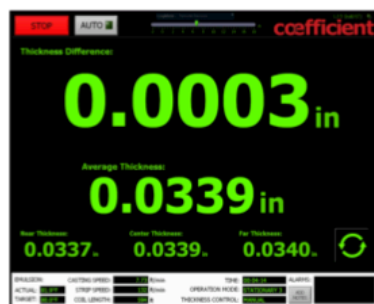
Large Numerical Display, Including Thickness Difference
